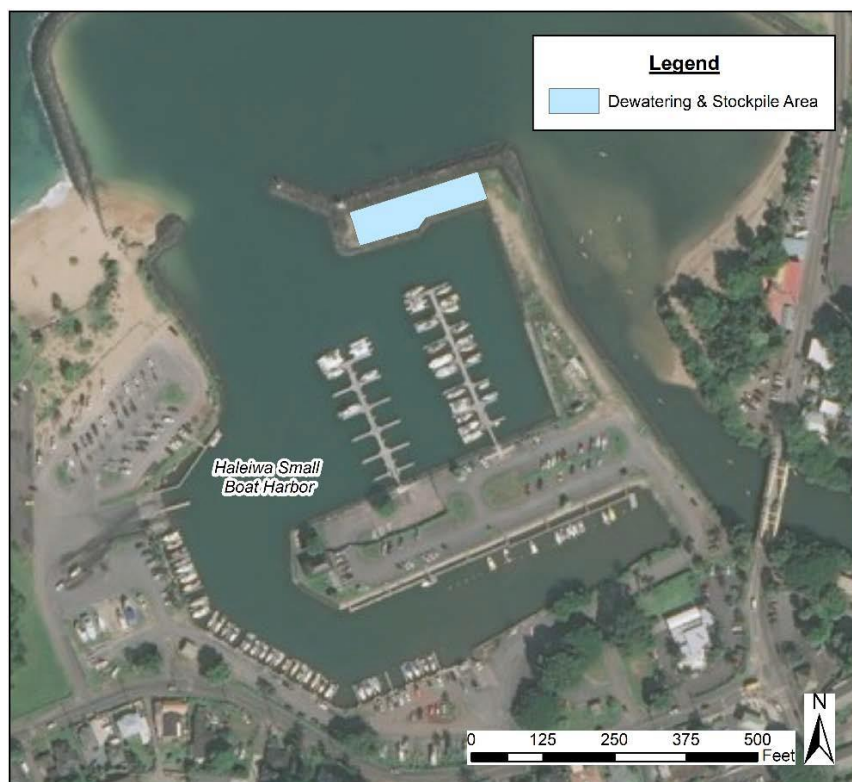
Figure 3. Location of stockpile area at Haleiwa Harbor during the 2009 maintenance dredging.
