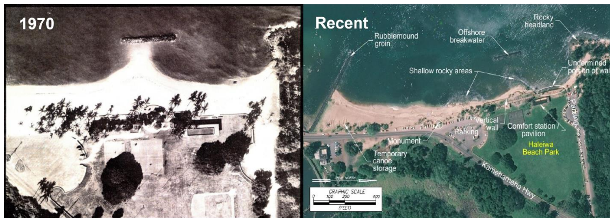
Figure 4. Photo of Hale'iwa Beach Park, circa 1970, Depicting the Historic Extent of Beach and Tombolo. (Sea Engineering Inc., 2019) Compared to Present day Conditions
